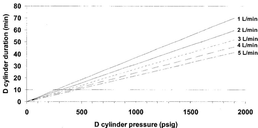
Figure 3. Estimated D cylinder duration in a low compliance (LC) 750 mL tidal volume with fresh gas flow of 1 to 5 L/min. Estimates extrapolated from data generated with the Narkomedâ M field anesthesia machine with a LC 750 mL tidal volume model and fresh gas flow of 1 L/min.
