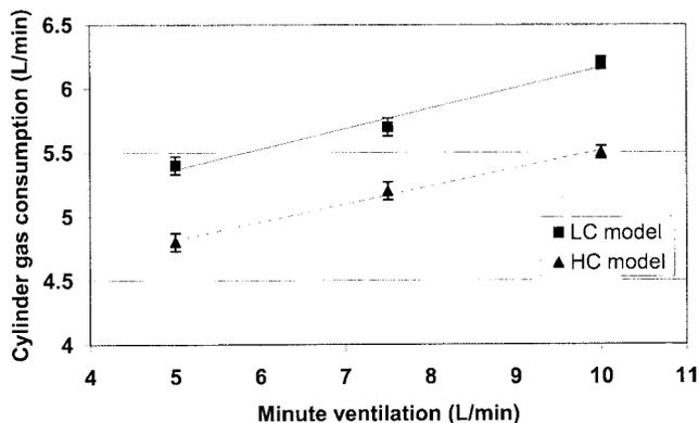
**Figure 1.** Cylinder gas consumption versus minute ventilation with fresh gas flow of 1 L/min. Results are means ± SD P < 0.001 for all same minute ventilation group comparisons, and P < 0.05 for all same lung model group comparisons. LC = low compliance, HC = high compliance.
