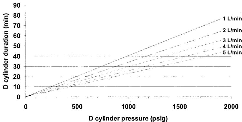
Figure 2. Estimated D cylinder duration in a high compliance (HC) 750 mL tidal volume with fresh gas flow of 1 to 5 L/min. Estimates extrapolated from data generated with the Narkomedâ M field anesthesia machine with a HC 750 mL tidal volume model and fresh gas flow of 1 L/min.
